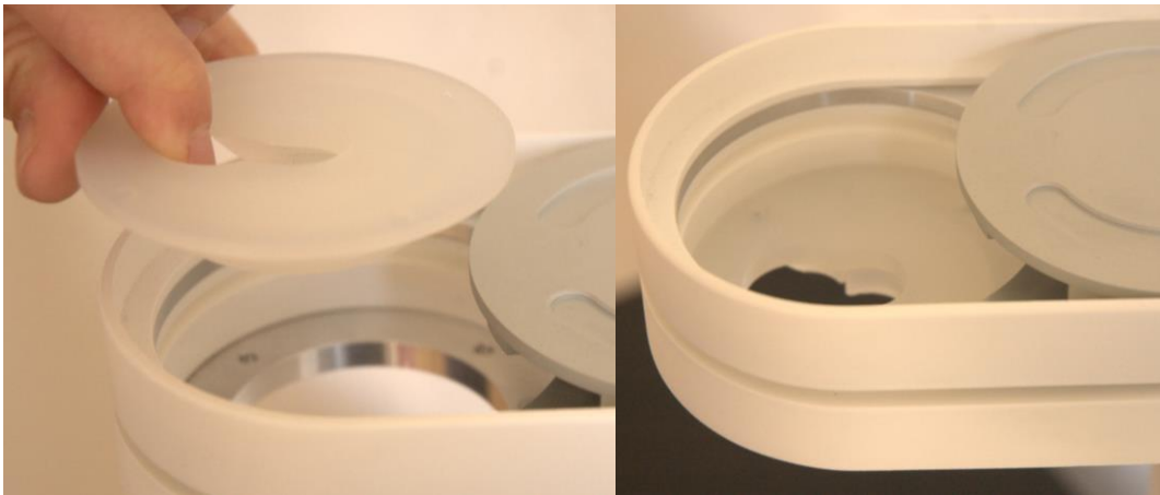
Figure 21: Insertion of the Bottom Part of the Adapter
