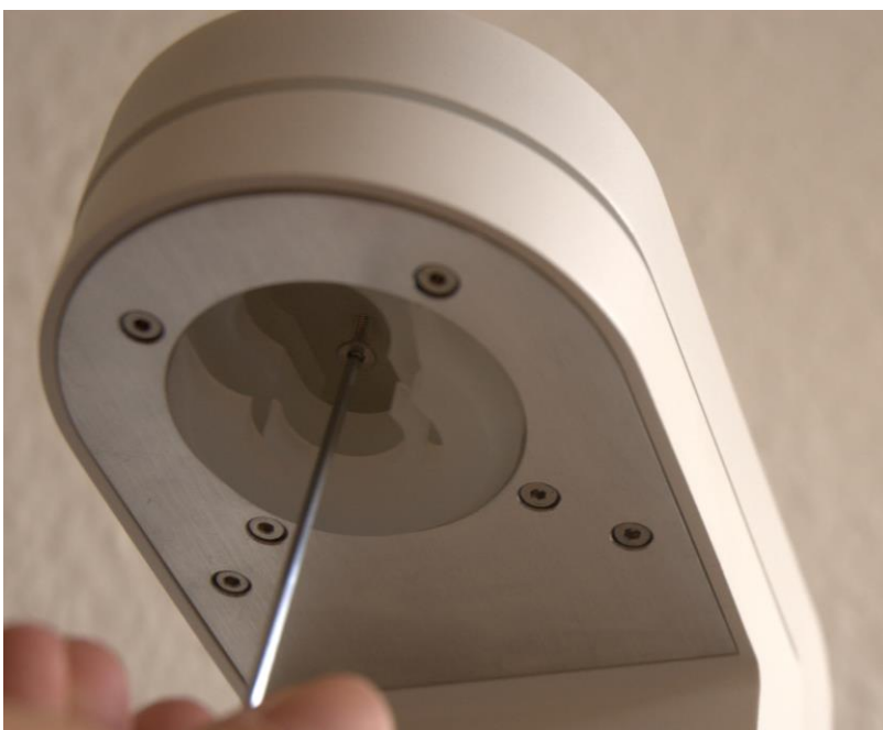
Figure 24: Tightening the Upper Part of the Adapter
