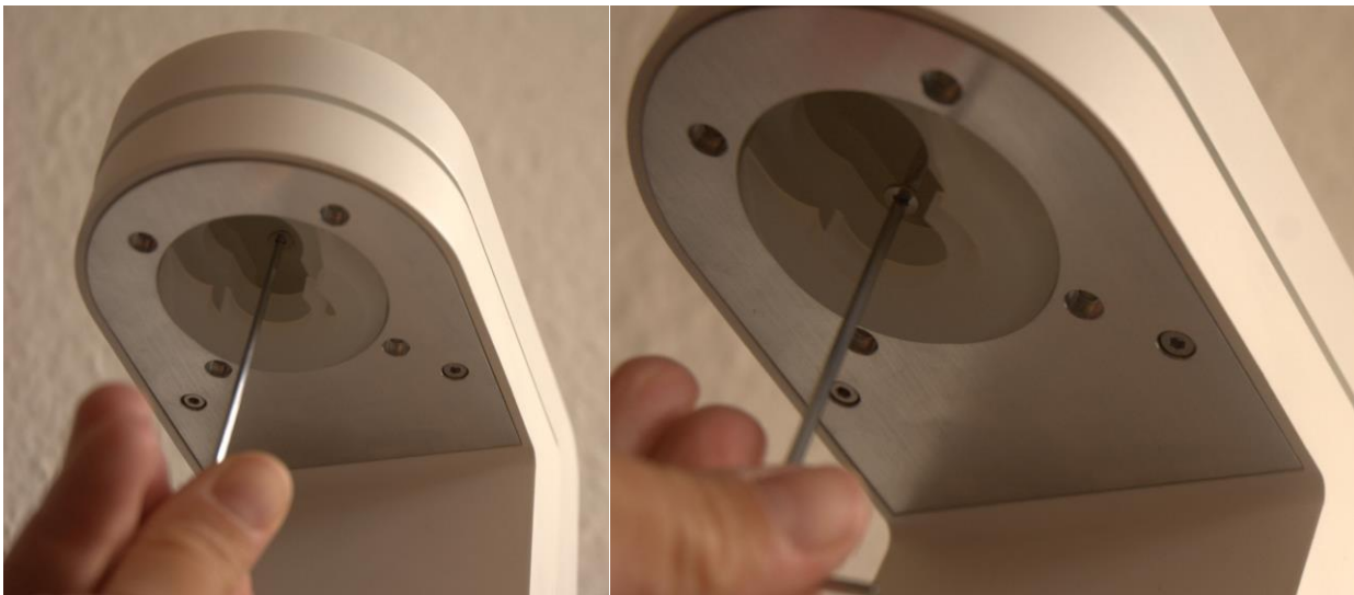
Figure 19: Unscrewing the Screws From the Upper Part of the Adapter
