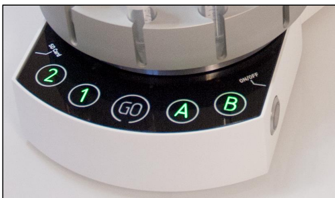
Figure 10 – Program Selection – Green Illuminated Keys
