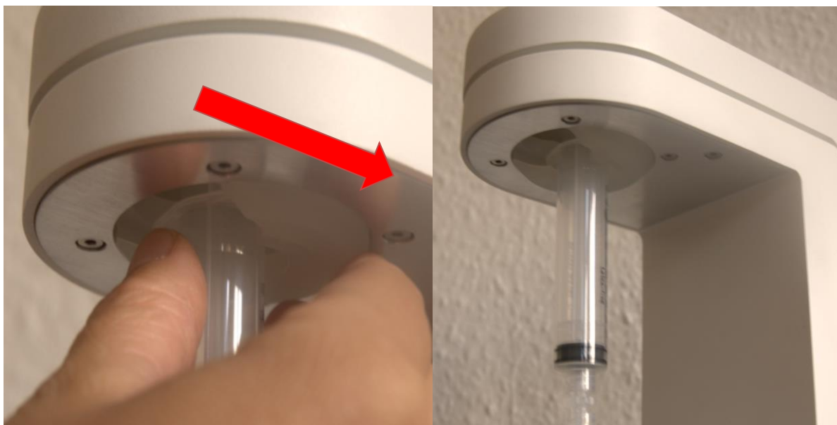
Figure 6: Insertion of the Syringe (2)
