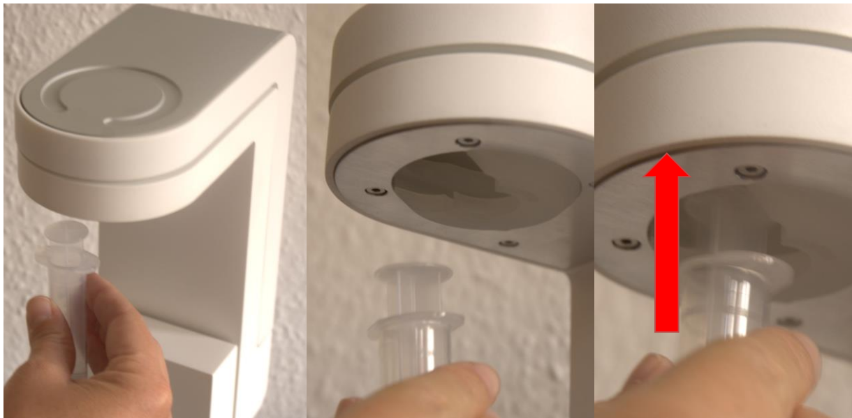
Figure 5: Insertion of the Syringe (1)
